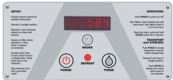
Figure 2: Phoenix R200 control board.
